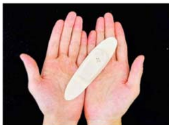
Disposable Holter ECG device "EG Holter"
